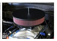
Test fit the air cleaner assembly (not included) onto the air cleaner stud to verify correct stud height (Fig. D1-D2). If needed, the air cleaner stud must be removed and cut to allow proper fitment of your specific air cleaner height or for hood clearance. (Fig. E1-E3)
